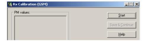
Set RF generator to required EGSM900 frequency => 0K.
